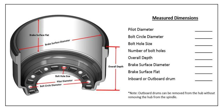
\*Verify the weight of the replacement brake drum is comparable to the weight of the brake drum being removed from the vehicle. If you have any questions, please visit Webb's Training Toolbox at <u>http://www.webbwheel.com/aftermarket/training\_toolbox.html</u> for additional information.
